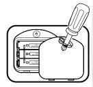
4. Replace the battery cover and tighten the screw to secure the battery cover.
